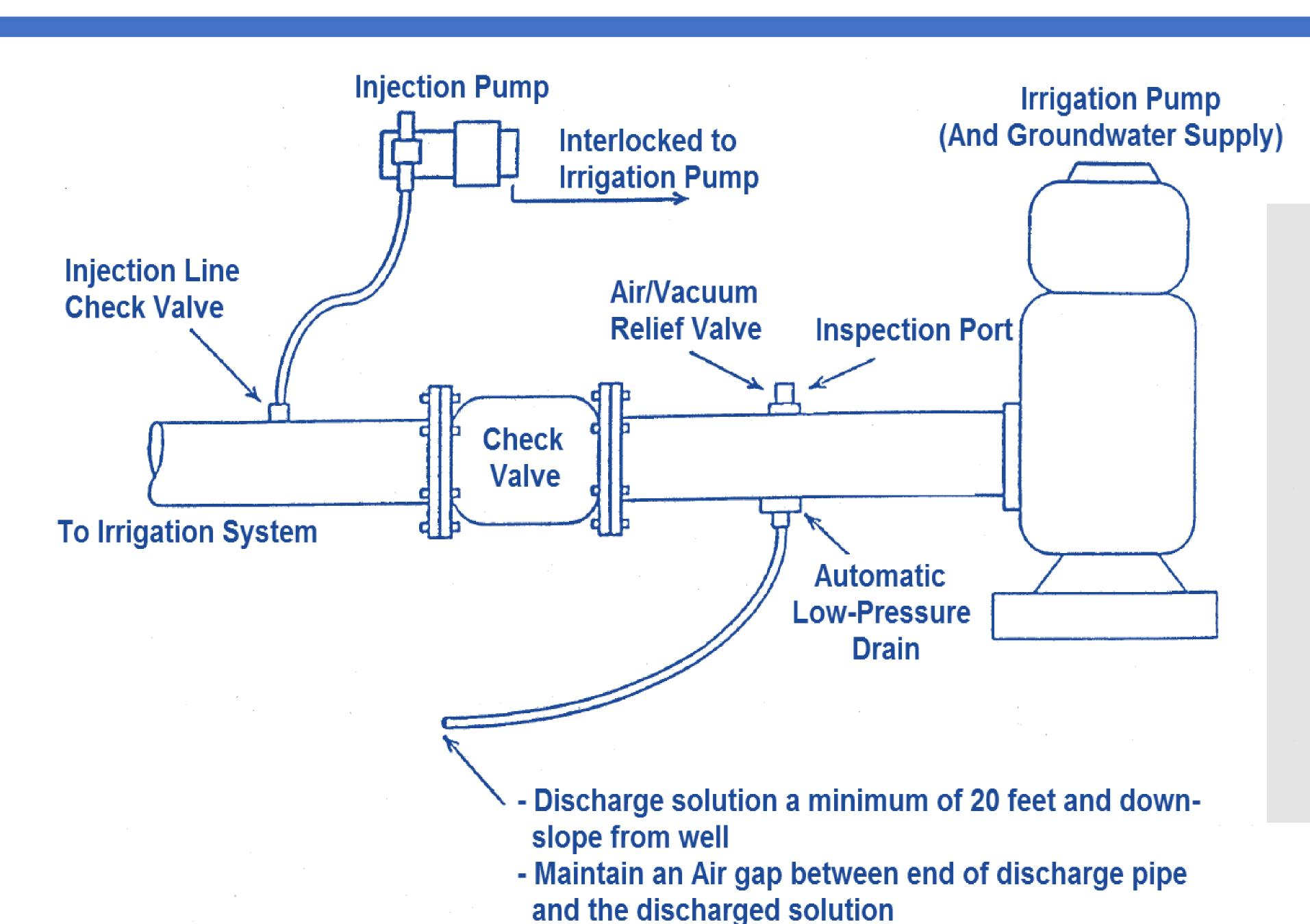
As shown in the diagram, effective backflow devices must include all the following:
