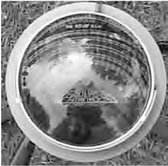
Figure 14-15. Trees and other shade producing features are reflected on the Solar Pathfinder dome. The transparent dome allows the user to see the sunpath diagram placed on the base of the instrument.
