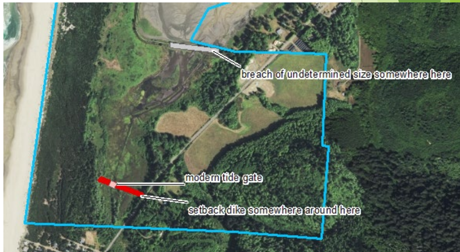
Setback dike - construct new dike closer to TDM that includes a modern tide gate, then breach the old dike... tide gate style/sizing/closure settings... location...
