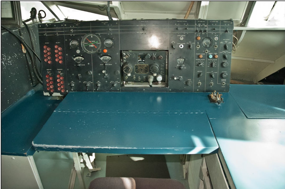
LOCATED ON THE H-4 HERCULES FLIGHT DECK, PORT SIDE, AFT OF PILOT'S POSITION, THE RADIO OPERATOR'S STATION FEATURES A MORSE CODE TELEGRAPH KEY IN FRONT OF THE PANEL, TO THE RIGHT.
