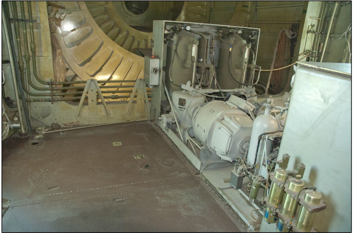
THE STANDBY HYDRAULIC STATION, LOCATED ON THE H-4 HERCULES CARGO DECK, NEAR THE NOSE. NOTE THE DURAMOLD FRAMEWORK OF THE NOSE, WITH ITS AGED SILVER-ALUMINUM PAINT DATING TO 1946-47 NOW A PATINA GREEN.
