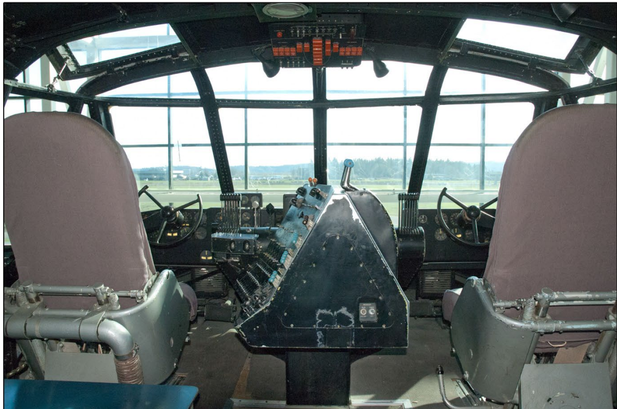
THE PILOT'S (LOCATED ON THE PORT SIDE) AND CO-PILOT'S (LOCATED ON THE STARBOARD SIDE) POSITIONS SIT ABOVE THE H-4 HERCULES NOSE ON THE FLIGHT DECK.
