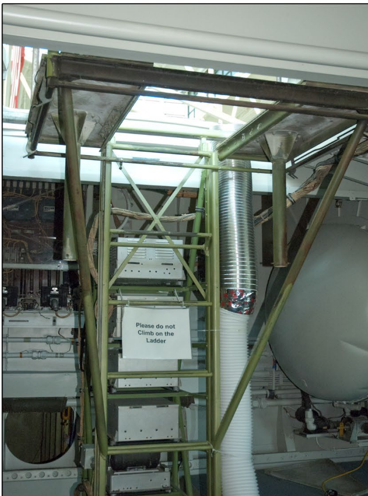
THE 281-GALLON OIL STORAGE TANK, SITS JUST OUTSIDE THE PORT SIDE LEADING EDGE WING ACCESS DOOR, AFT, ON THE H-4 HERCULES FLIGHT DECK.
