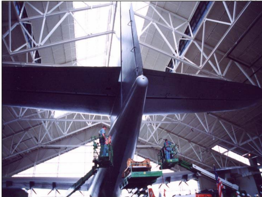
H-4 HERCULES - AFTER INSTALLATION OF THE CONTROL SURFACES, TAIL CONE ASSEMBLY TOOK PLACE ON DECEMBER 7, 2001.
