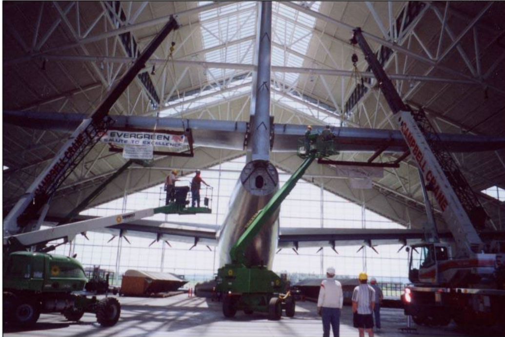
H-4 HERCULES - WITH WINGS, ENGINES AND PROPELLERS, VERTICAL AND HORIZONTAL STABILIZERS ASSEMBLED, 2001.
