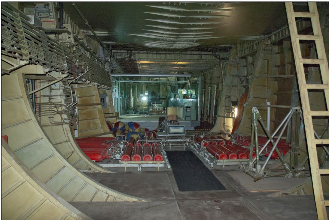
THE H-4 HERCULES INTERIOR, CARGO DECK LOOKING FORWARD TOWARD VIEWING CUBE. NOTE THE 36 RED CO 2 PRESSURE TANKS AT THE CENTER, AND THE HYDRAULIC TUBING TRAVELING DOWN ON THE PORT SIDE.
