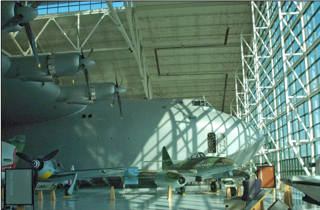
THE NOSE OF THE H-4 HERCULES FACES SOUTH WITH THREE OF THE PRATT AND WHITNEY R-4360 ENGINES SHOWING ON THE STARBOARD WING, EACH FEATURING HAMILTON STANDARD PROPELLERS.
