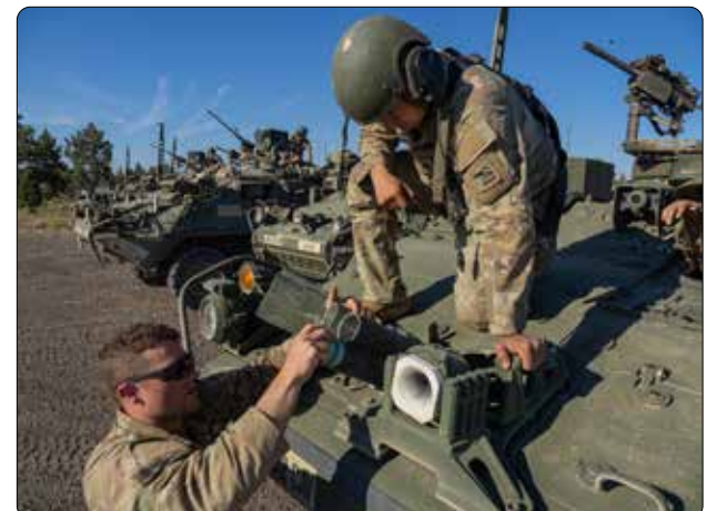
Sgt. Steven South (left) and Sgt. Tyler Hanish of A Troop, 1st Squadron, 82nd Cavalry, load smoke grenades onto an M1127 Reconnaissance Vehicle Stryker during training on June 22, 2024.
