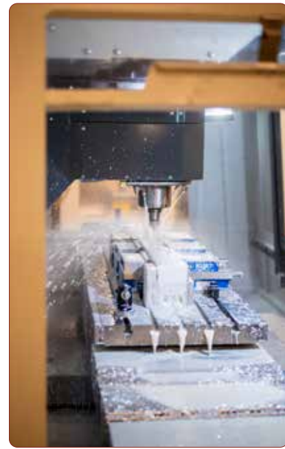
A Computer Numerical Control Mill housed within the 142nd Wing's fabrication flight shop cuts metal into an essential part for the F-15C Eagle.
