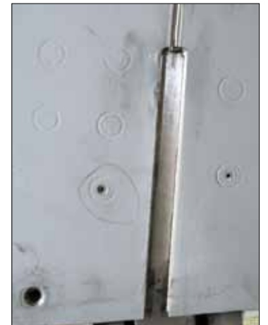
Seen from below, the cutting opens a 5-inch by 1/2-inch wide section of titanium skin, which allows for the non-destructive inspection shop to examine the underlying wing spar. It will remain open and has no effect on any other part.
