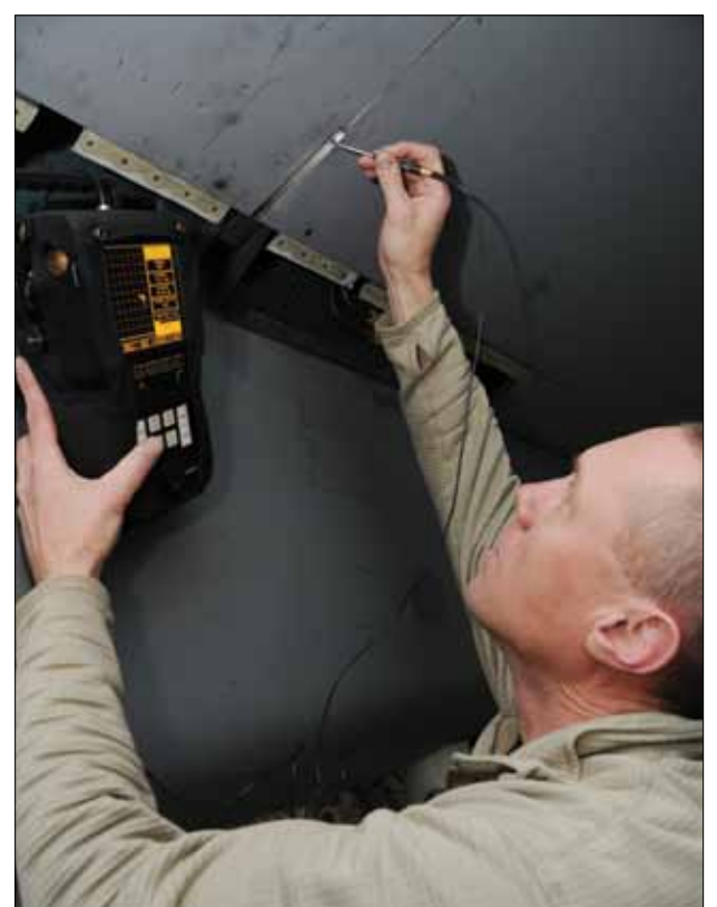
Tech. Sgt. Peter McNally, of the non-destructive inspection shop, uses an Eddy Current Tester inside the skin opening to scan the wing spar for cracks.
