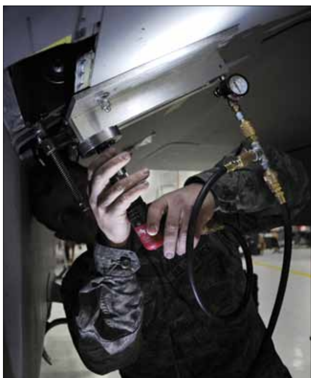
Childs’ fixture, seen at the top of the photo, keeps the bit steady while he makes the most crucial final pass where it’s possible to unintentionally cut into the wing spar itself. He holds the drill lightly with both hands where he can sense even the slightest change in vibration to avoid the spar.
