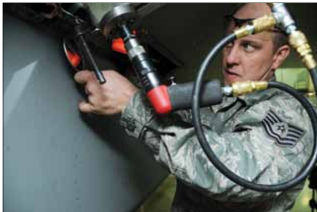
Tech. Sgt. Jeff Childs, with the 173rd Fighter Wing sheet metals shop, requires a small mirror to help ensure his cutting tool does not cut the wing spar while taking fine cuts, measuring only a thousandth of an inch, on the skin of an F-15 aircraft wing. While removing the quarter-inch of titanium skin covering the wing, the delicate part is ensuring he does not damage the underlying spar.
