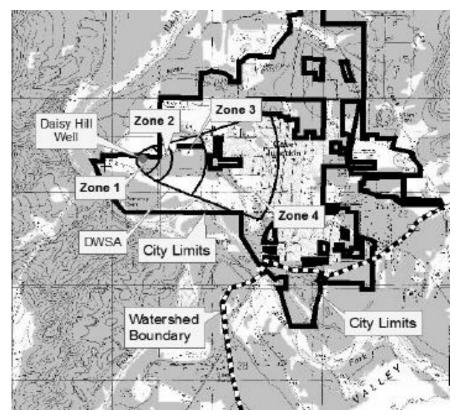
Figure 1. The Drinking Water Protection Area for the city of Cave Junction's Daisy Hill Well. Boundaries are marked for the 1-, 2-, 5- and 10-year time-of-travel for groundwater to move through the aquifer to the well. Also shown are the city limits and the watershed boundary near the city's intake.
