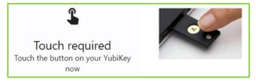
16. Once the YubiKey hardware token is touched, a six-digit code is visible on the Yubico Authenticator. Click on the **Copy icon** which will copy to clipboard. This code is valid for up to 30 seconds.
