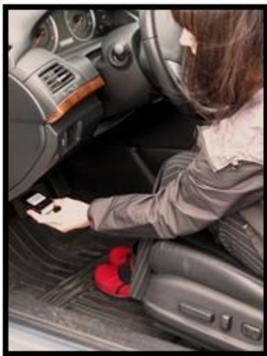
Figure 5: Installation of an OBD-based MRD
