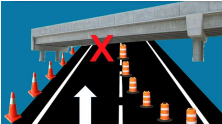
Figure 7: A lane closure/lane shift under a structure can result in lower vertical clearance
