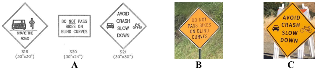
Figure 2.4: Mount Diablo State Park Signage: (A) Engineering Drawings for Signs S19-21, Source: (Trujillo, 2016); (B) Sign S20; (C) Sign S21, Source: ("Our Story," n.d.)
