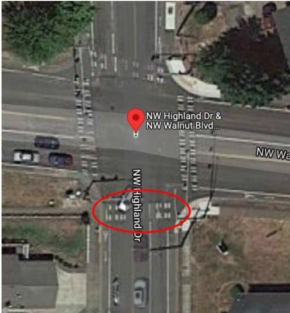
Setback (highlighted in red) crosswalk at NW Highland Dr. and NW Walnut Blvd.
