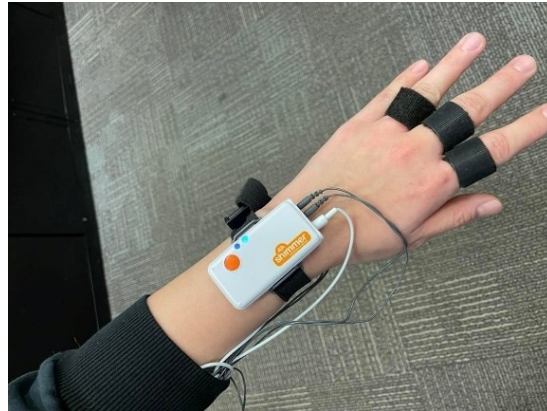
Figure 4.5: Shimmer3 SGR+ sensor strapped to participant's wrist
