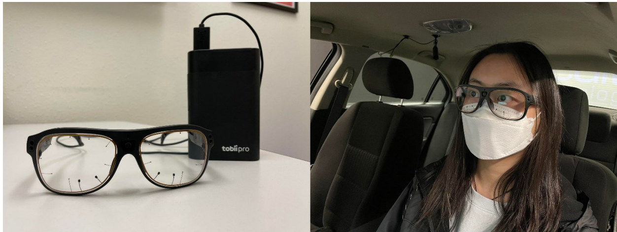
Figure 4.4: Tobii Pro Glasses 3 (left) and OSU researcher demonstration in the driving simulator (right)
