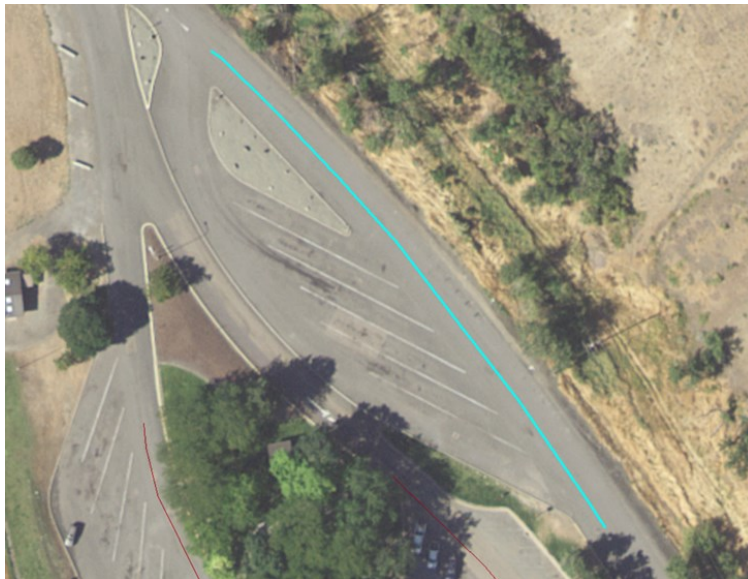
Figure 3.27: Example of location with large shoulder width due to side-of-the-road parking
