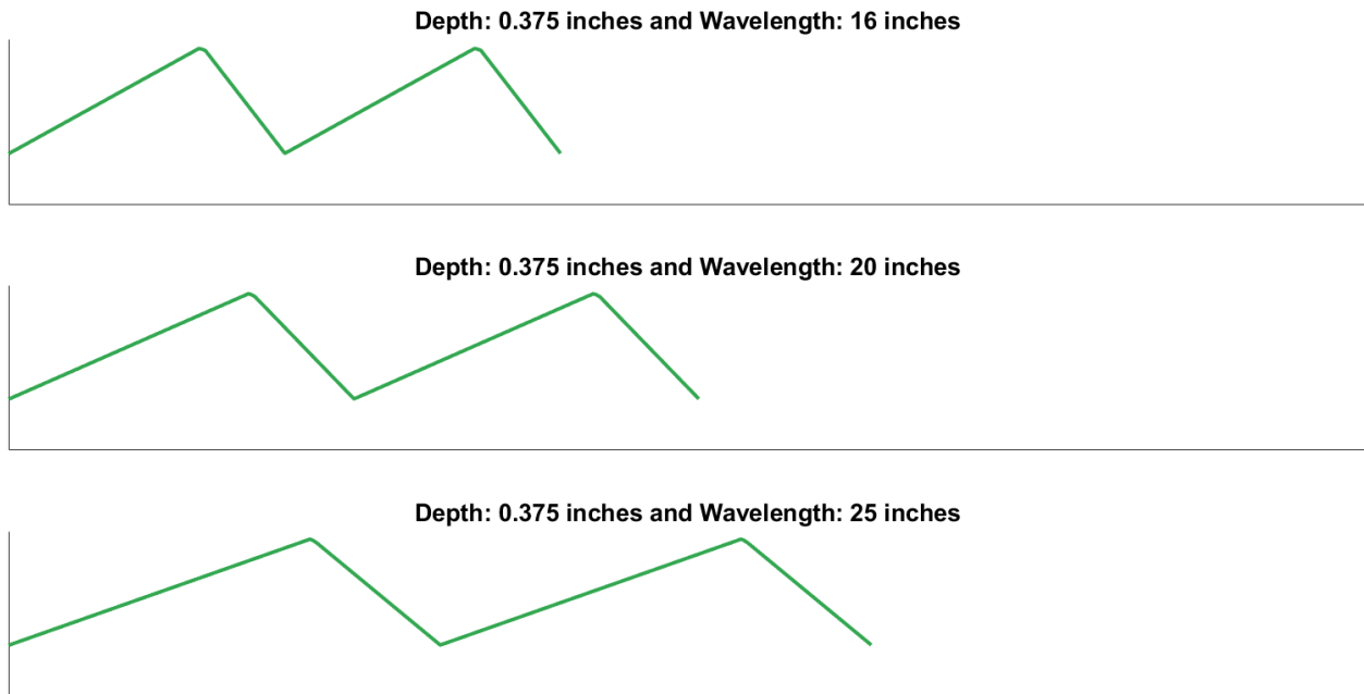
Figure 5.2: Side profiles of the sawtooth-short-climb-slow-drop design.
