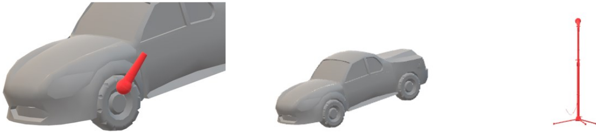
Figure A.4: Positions for microphones/sound level meters (colored in red) for exterior sound level measurements.
