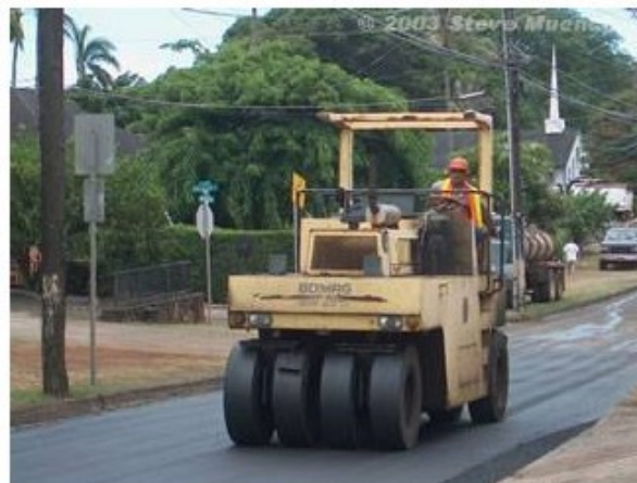
Figure 2.17. Pneumatic tire Roller (Source: www.pavementinteractive.org )
