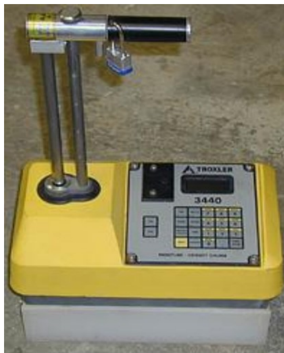
Figure 2.30. Nuclear density gauge (Schwartz et al. 2014)
