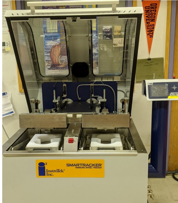
Figure 3.5. Hamburg wheel tracking device (HWTT) at the OSU Asphalt Materials Performance Lab.
