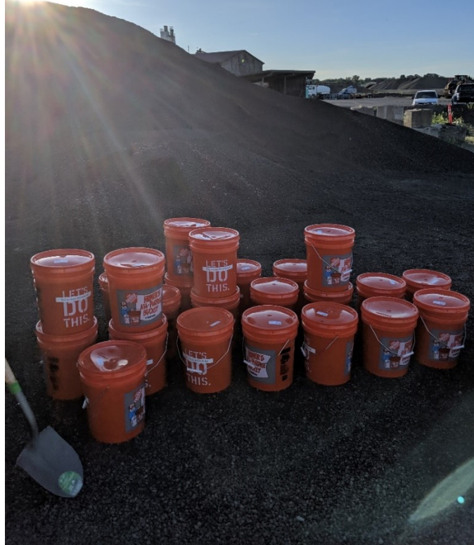
Figure 3.1. RAP material sampled from the plant
