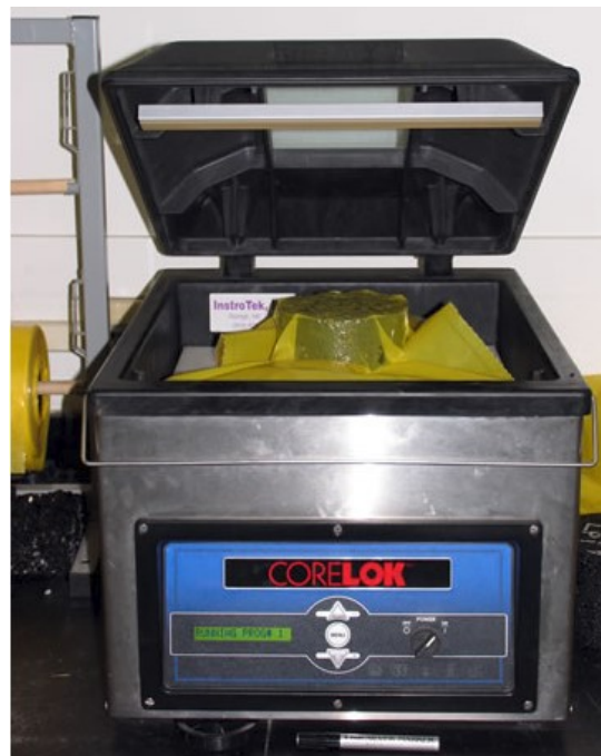
Figure 2.29. CoreLok vacuum chamber (Source: www.pavementinteractive.org )
