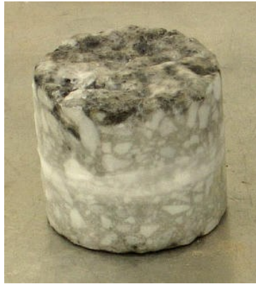
Figure 2.26. Paraffin-covered HMA specimen (Source: www.pavementinteractive.org )
