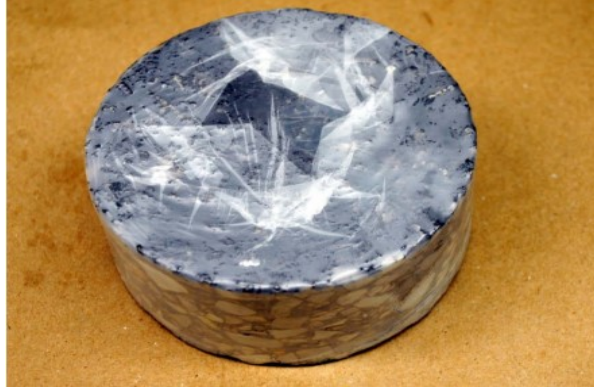
Figure 2.27. HMA specimen covered with Parafilm (Schroer 2012)
