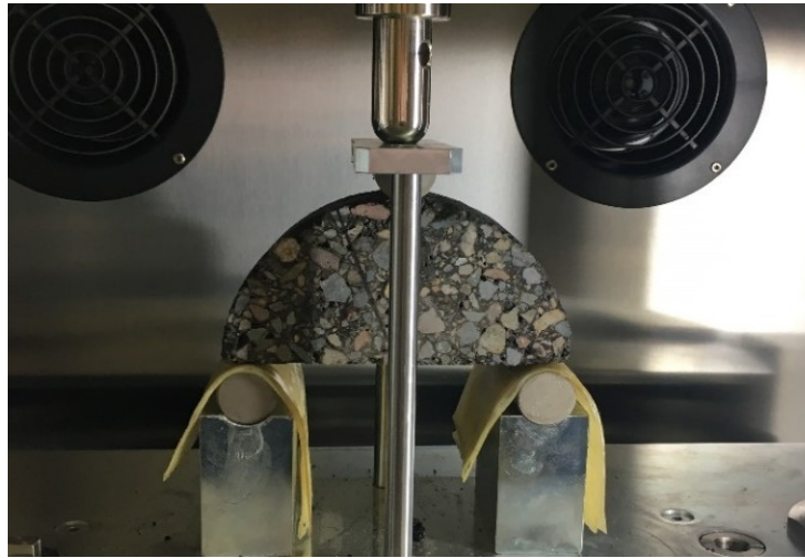
Figure 3.3. SCB test up
