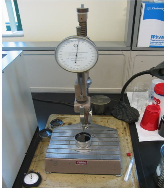
Figure 2.9. Penetration test apparatus used for penetration grading (Source: www.pavementinteractive.org )
