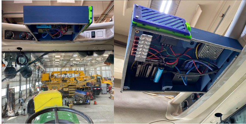
Figure 4.3: Prototype hardware enclosure, mounted to radio deck bracket
