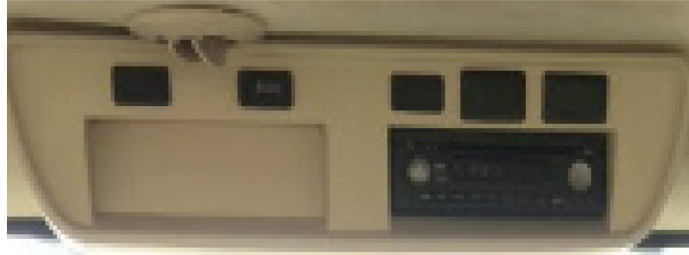
Figure 3.2: Electrical Accessory Slot
