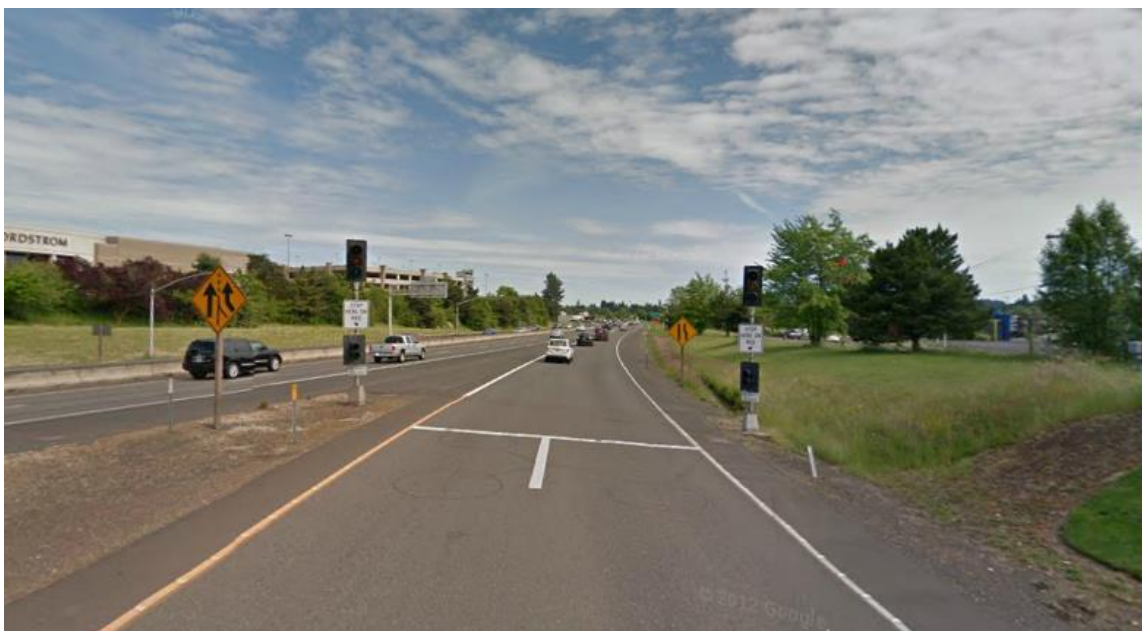
Figure 13-6 |Ramp Meter Signal Assembly Example – Controlling Two Lanes of Traffic
