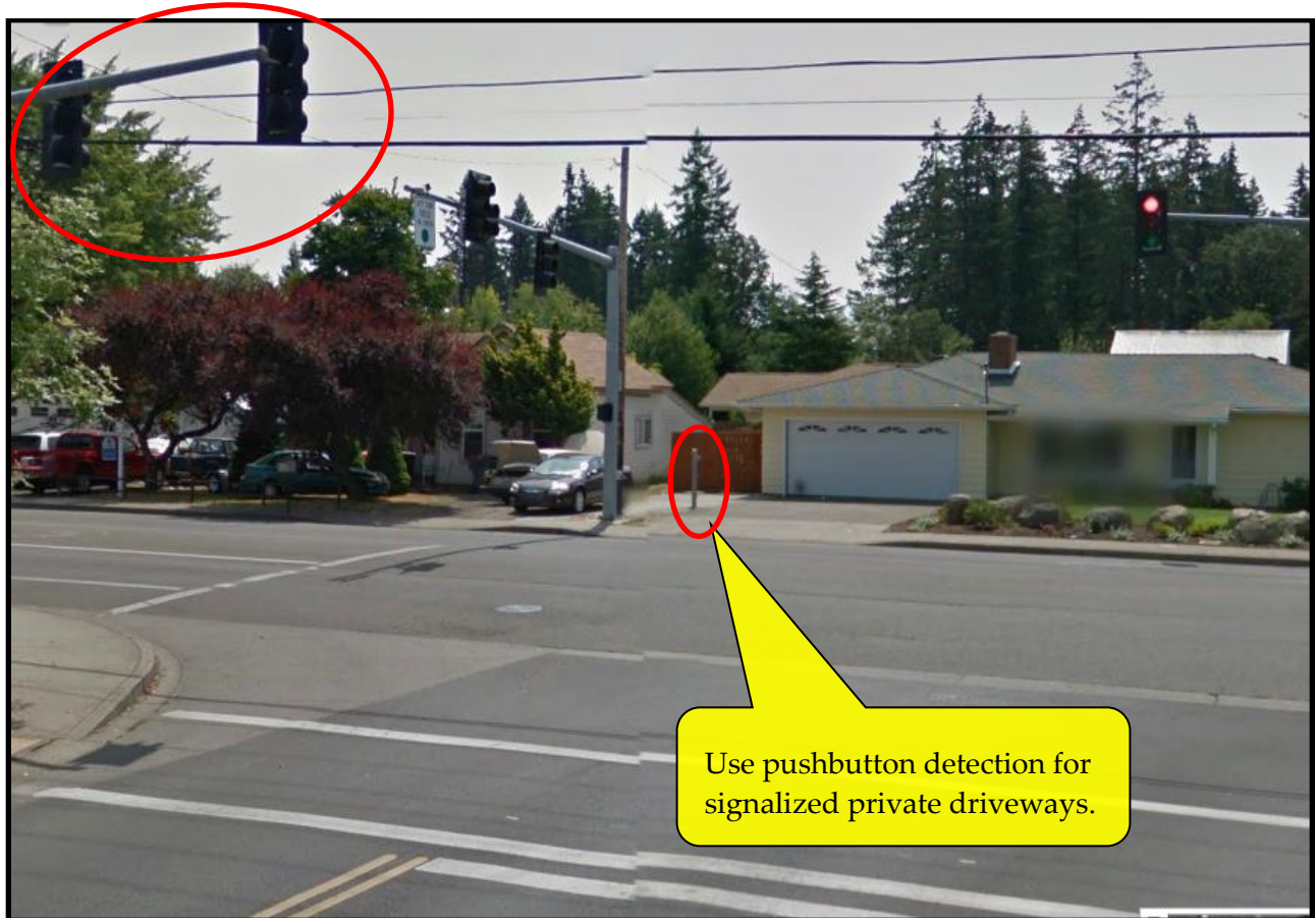
Figure 6-9 | Detection Placement Considerations: Private Driveway Signalized Approaches
