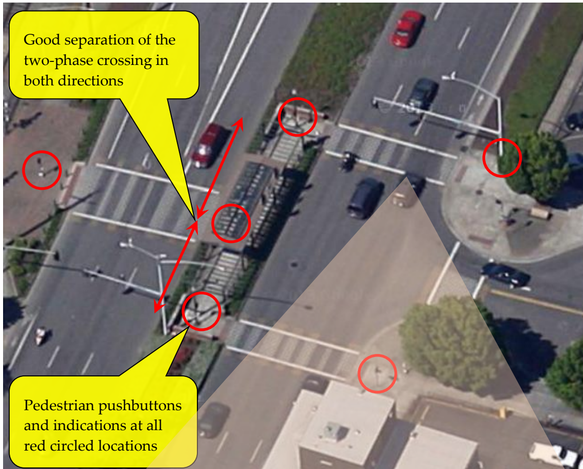
Figure 5-9 | Two-Phase Pedestrian Crossing (Staggered Crosswalk Alignment) Example 1
