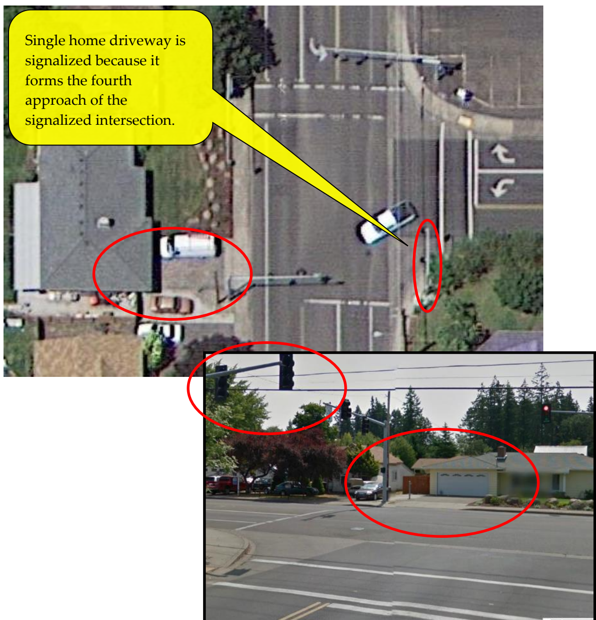
Figure 5-15 | Signalized Driveway Example
