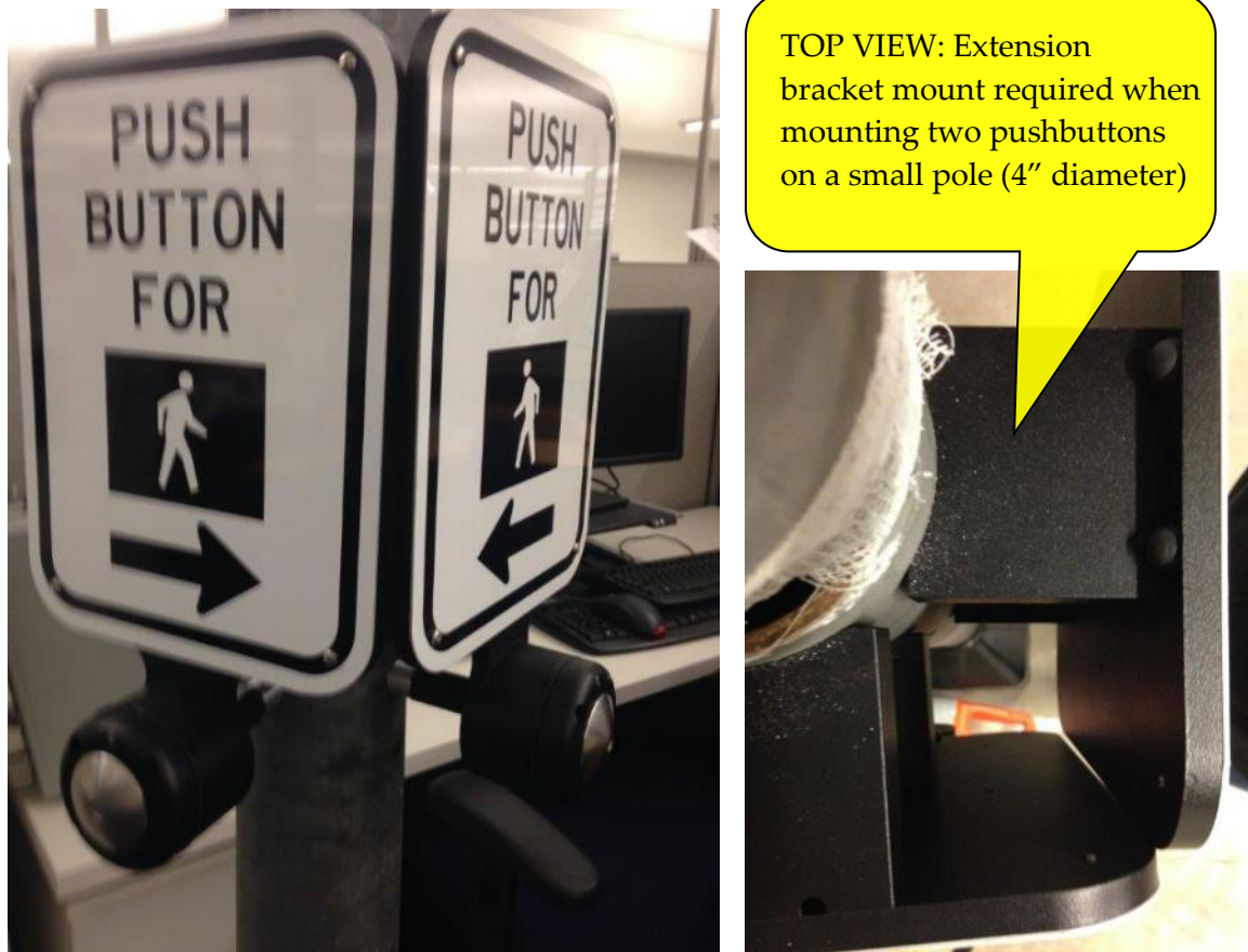
Figure 5-91 | Extension Bracket Mount for Two Pushbuttons on 4 Inch Diameter Pole
