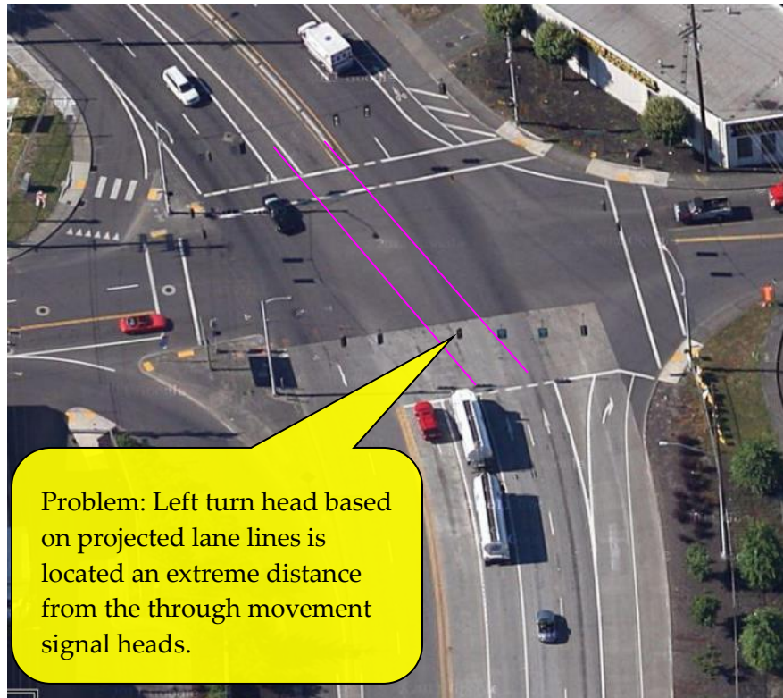
Figure 5-32 | Horizontal Curves and Signal Head Alignment, Example 2
