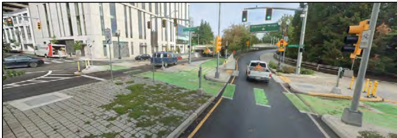
66 67 Figure 8: Bicycle Signal Controlling Separated Bicycle Lanes, Markings and Geometry Showing 68 Allowable Movements
