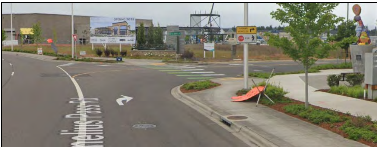
71 Figure 7: Separated Bicycle Lane (curb-separated) to the Right of a Right Turn Lane (right-in- 72 right-out)
