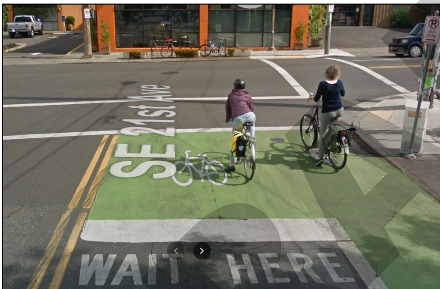
51 52 Figure 4: Bicyclist Using Proposed Detector Marking in Bicycle Box
