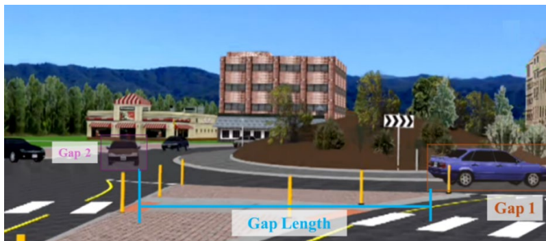
Figure 41: Example of Gap Vehicles and Gap Length Measurement in Driving Simulator
