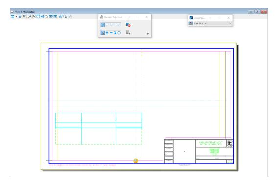
The named boundary is centered on the sheet and not correctly positioned within the border. Use the snapping points available from the *borderfull* cell to move the reference into its correct position in the sheet.
