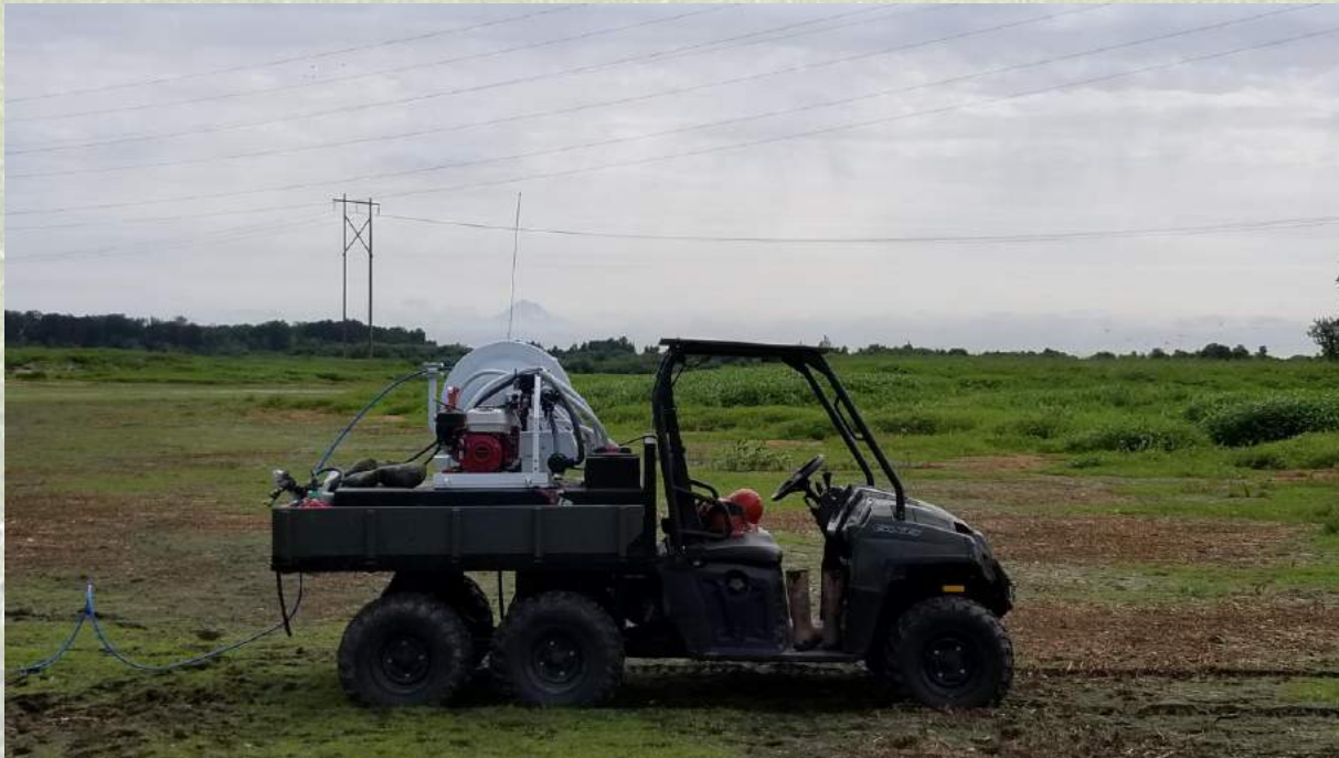
6x6 UTV Intelli-Spray with 100 gallon tank and 700' of hose
