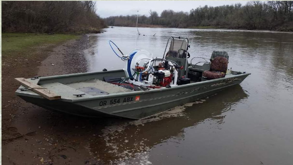
100 gallon Intelli-Spray mounted in jet boat
