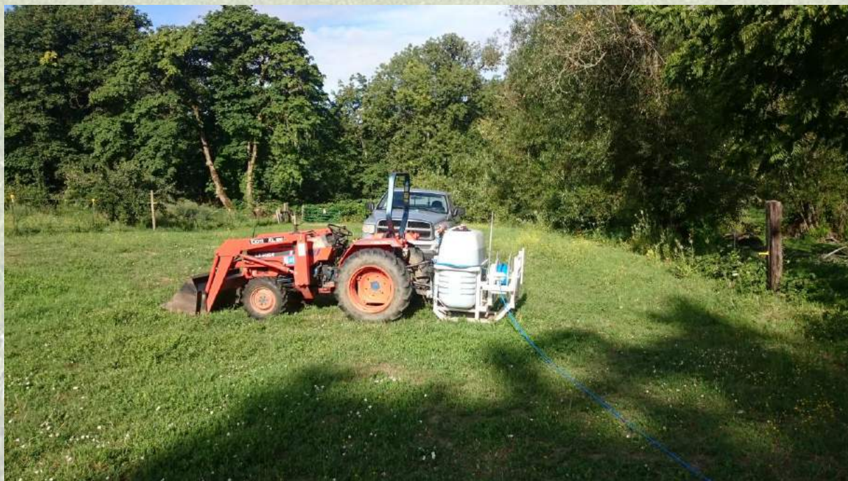
Tractor mounted Intelli-Spray with 120 gallon tank and 700' of hose
