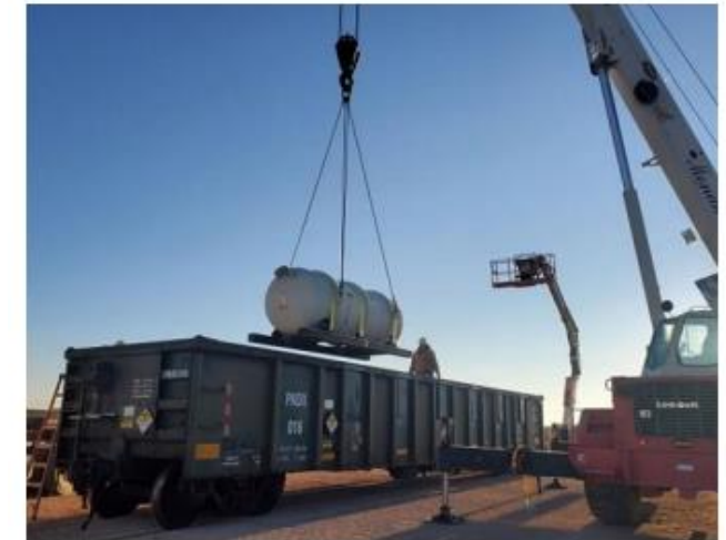
Figure H-32. Gondola Car from Portsmouth Site being Unloaded at Waste Control Specialists
