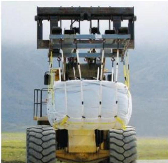
Figure H-28. Example of Soft Side Container for Shipping Low Specific Activity Materials
