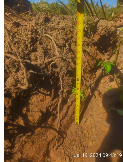
The 1.5-ft sample depth being measured in a test pit.
