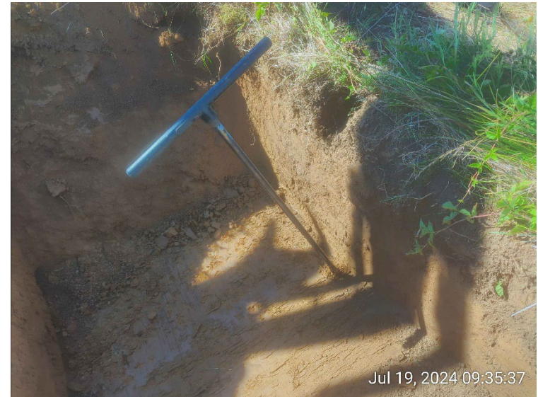
Sampling at the 2.5-foot depth interval in a test pit. The 2.5-ft sample was held pending results of the shallower samples.
