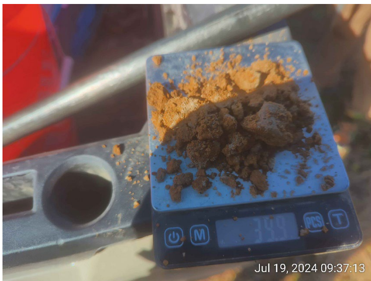
Sixty (60) soil increments, each weighing approximately 40 grams, were collected at each depth interval.
