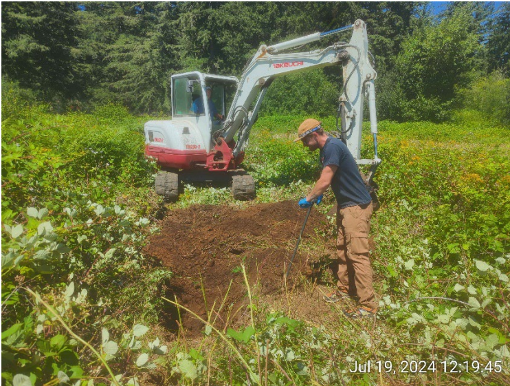
Using a decontaminated stainless-steel hand auger, soil increments were collected at 0.5-ft (shown here), 1.5-ft, and 2.5-ft. Two sample replicates (Rep01 and Rep02) were collected at 0.5-ft.
