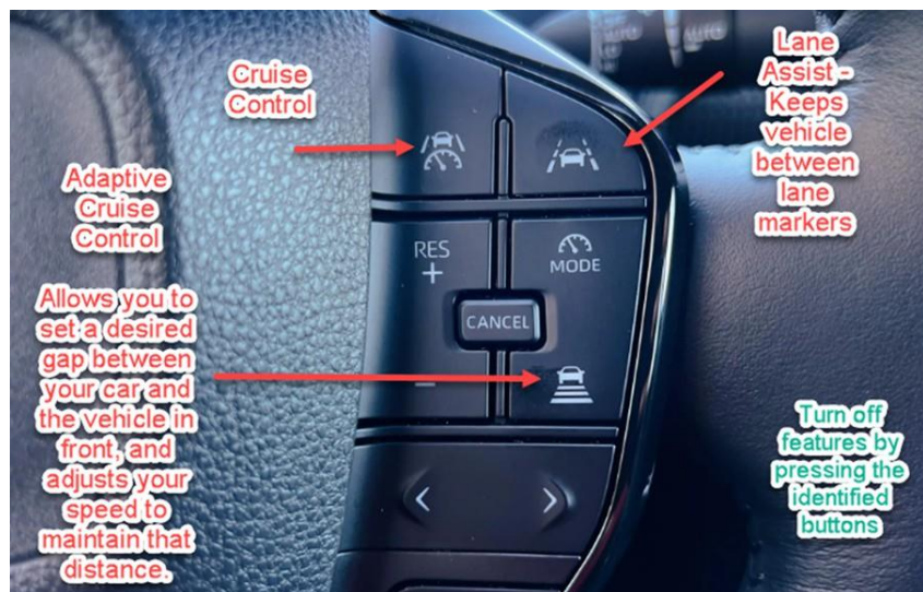
An example of how to turn off Lane Assist or Adaptive Cruise Control features. Your vehicle's icons may look different.
