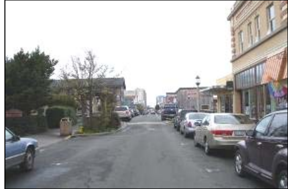
Figure 14: Downtown Seaside with Pedestrian Amenities – Curb Extensions, Street Trees, Pedestrian-Scale Lighting, Stamped Crosswalk, Trash Cans – Improves the Pedestrian Experience
