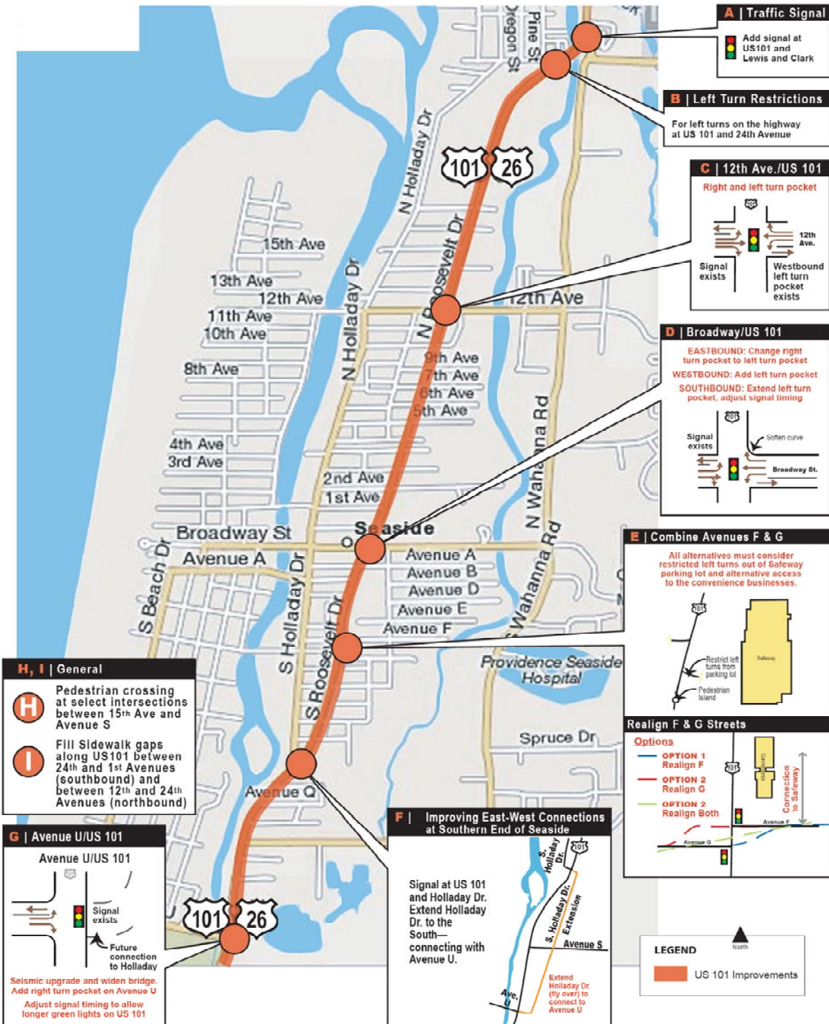
Figure 4: Roadway Improvements on US 101
