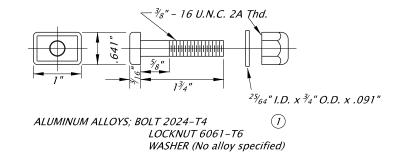
POST CLIP BOLT, NUT, & WASHER DETAIL
