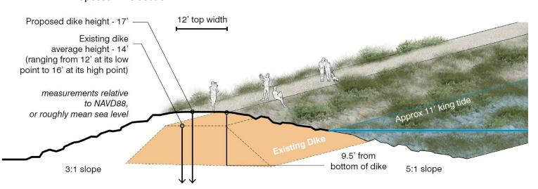
\* The existing dike is shown nested under the proposed dike only for size and elevation comparison. The proposed dike will be constructed in a different location than the existing.
