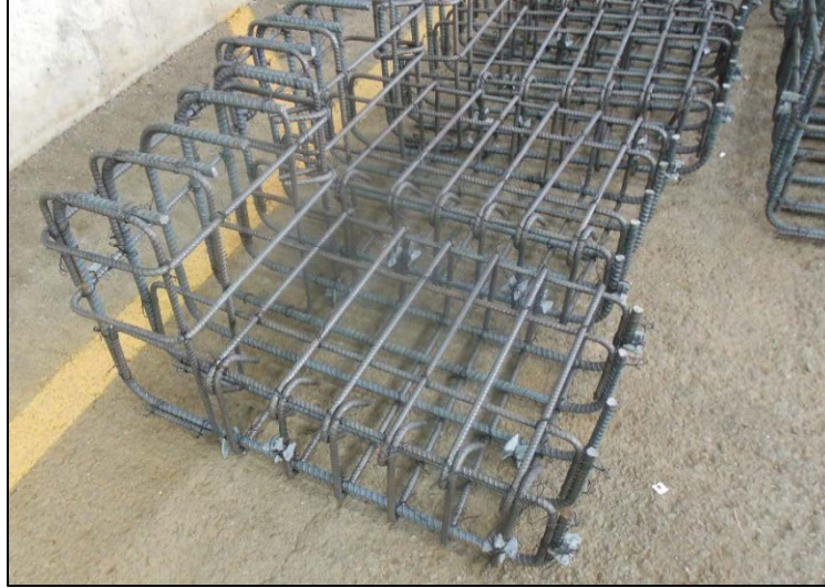
Figure 3.19: Reinforcing cage for a specimen containing #5 (#16M) reinforcing bars across the interface
