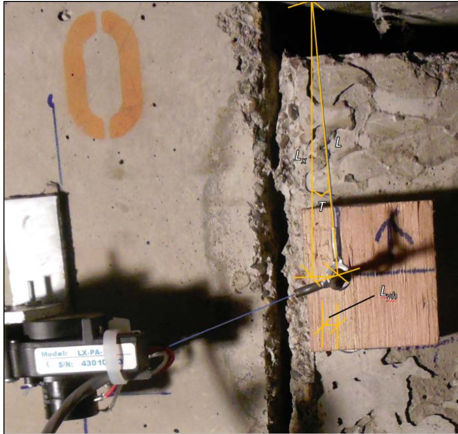
Figure 3.27: Vertical interface string potentiometer correction
