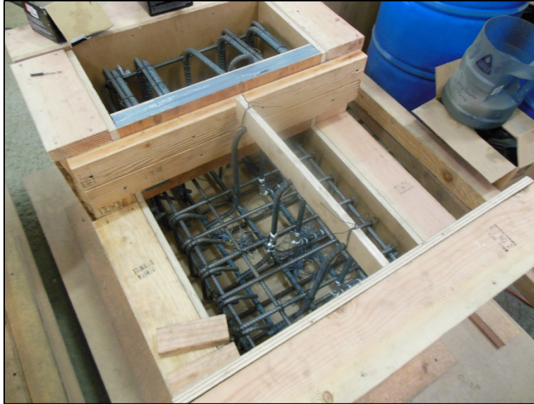
Figure 3.21: Specimen prepared for the first concrete cast
