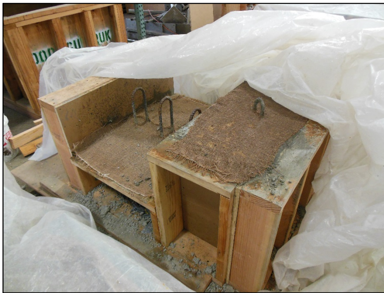
Figure 3.22: The L-shape half of a specimen containing #5 (#16M) reinforcing bars across the interface after the first concrete cast
