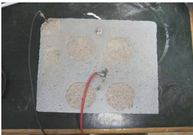
Figure 3.5: Example of electrochemically aged block used for resistance measurements
