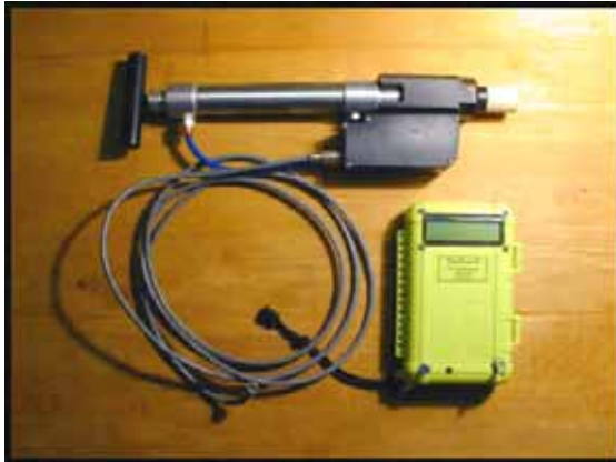
Figure A.2: The TinyPerm can be operated by one person and easily carried in a small backpack. The unit is weather and dust resistant and comes in a rugged case for transportation and shipping. The micro-controller and electronics are enclosed in a sturdy weatherproof case with LCD display, operating continuously for several hours on a single 9-volt alkaline battery ( Vindium 2006 ).
