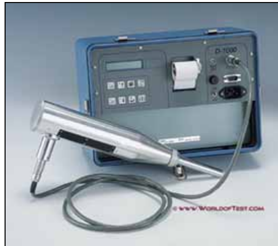
Figure A.11: Digital Model W-D-1000 which is an advanced, completely automated digital test hammer. Its calculation, memory and recording functions allow for quick, easy and accurate test results ( Qualitest 2006 )
