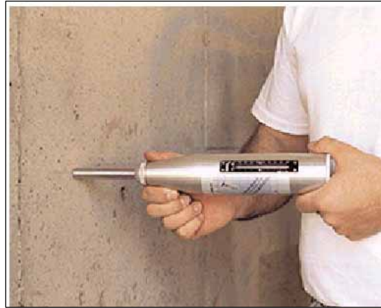
Figure A.10: Schmidt hammer being used in the field to measure the compressive strength of the concrete ( Cement Association of Canada 2006 )
