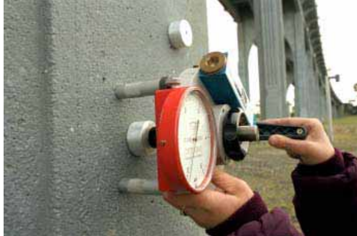
Figure A.16: Proceq portable tester used to measure the bond strength of the Zn anode on concrete (Covino, et al. 2002)
