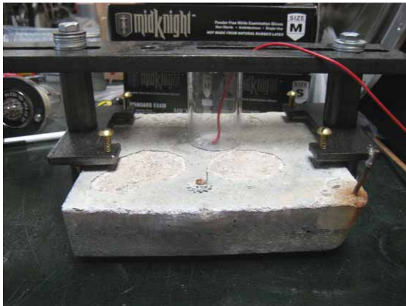
Figure 3.6: Device used in wet resistance measurements
