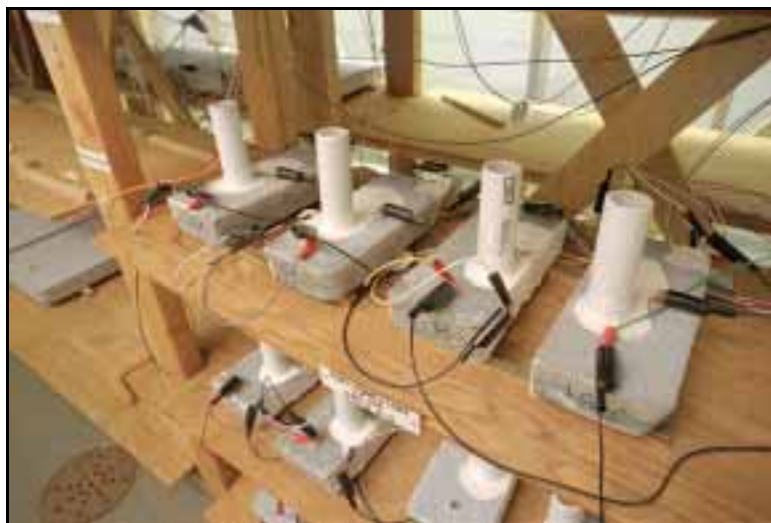
Figure 4.3: Aged zinc slabs wired in series in the high RH enclosure. Note the reference electrode holders (PVC pipe) mounted in areas without zinc left from prior adhesion strength pull tests.
