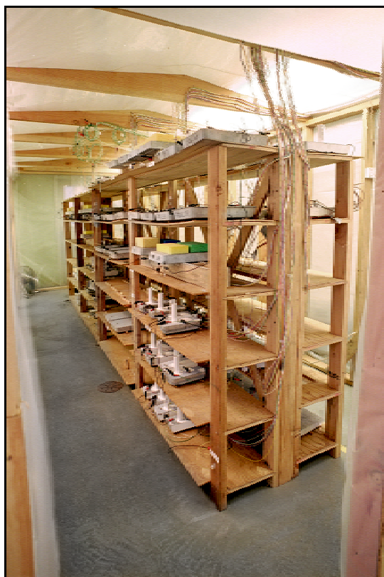
Figure 4.2: New and aged zinc slabs wired in series in the high RH enclosure
