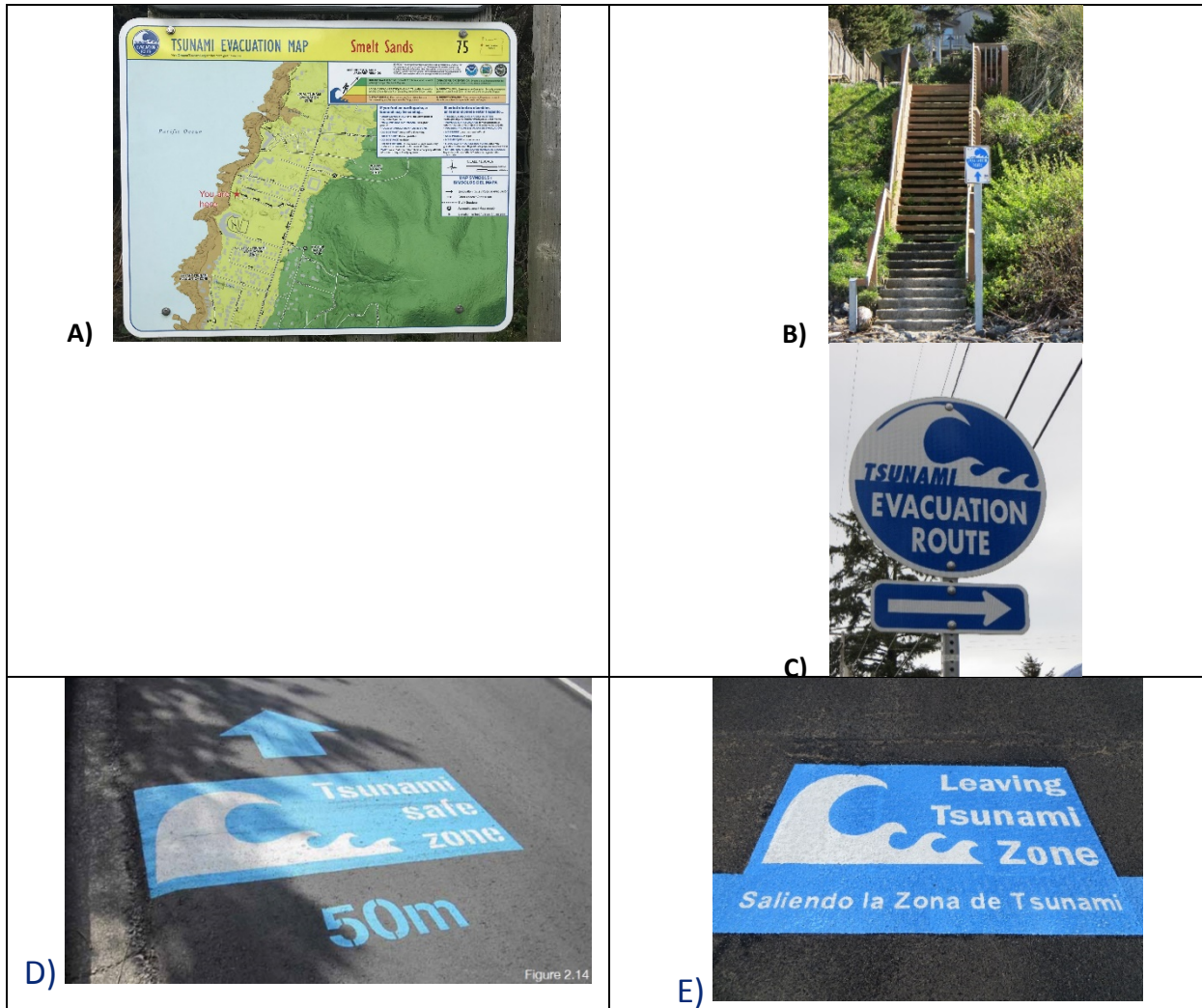
Figure 1. An end-to-end evacuation route plan consists of (A) 'You are here' signage and route guidance for high traffic sites; (B) Guidance signage established at the start of the route used in Cannon Beach and visible from the beach, as well as signage on posts along the route (C). Signage may also be painted on roads or footpaths with distance to safety identified (D). Finally, signage indicating that you have reached your safety destination (escape point) and have left the inundation zone needs to be identified along every evacuation route (E).
