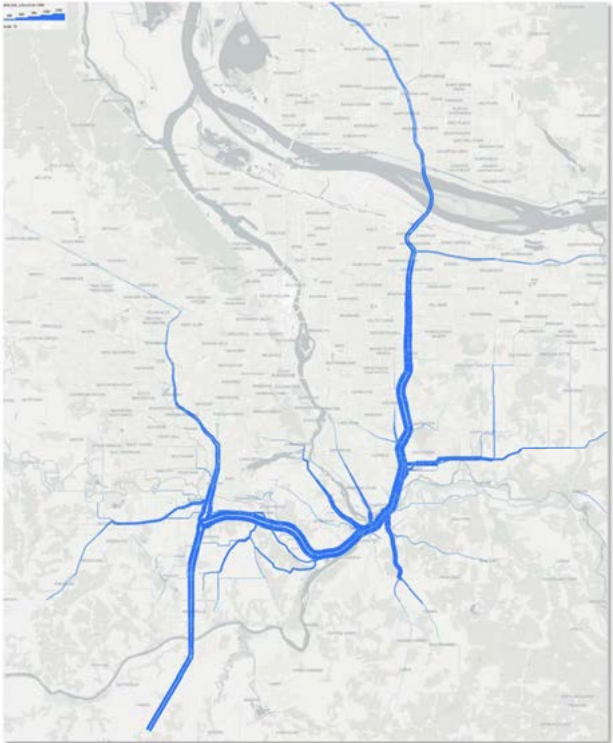
Figure 6 - 2045 Build PM Peak Traffic Select Link Analysis for the I-205 Bridge – Wider Model Context
