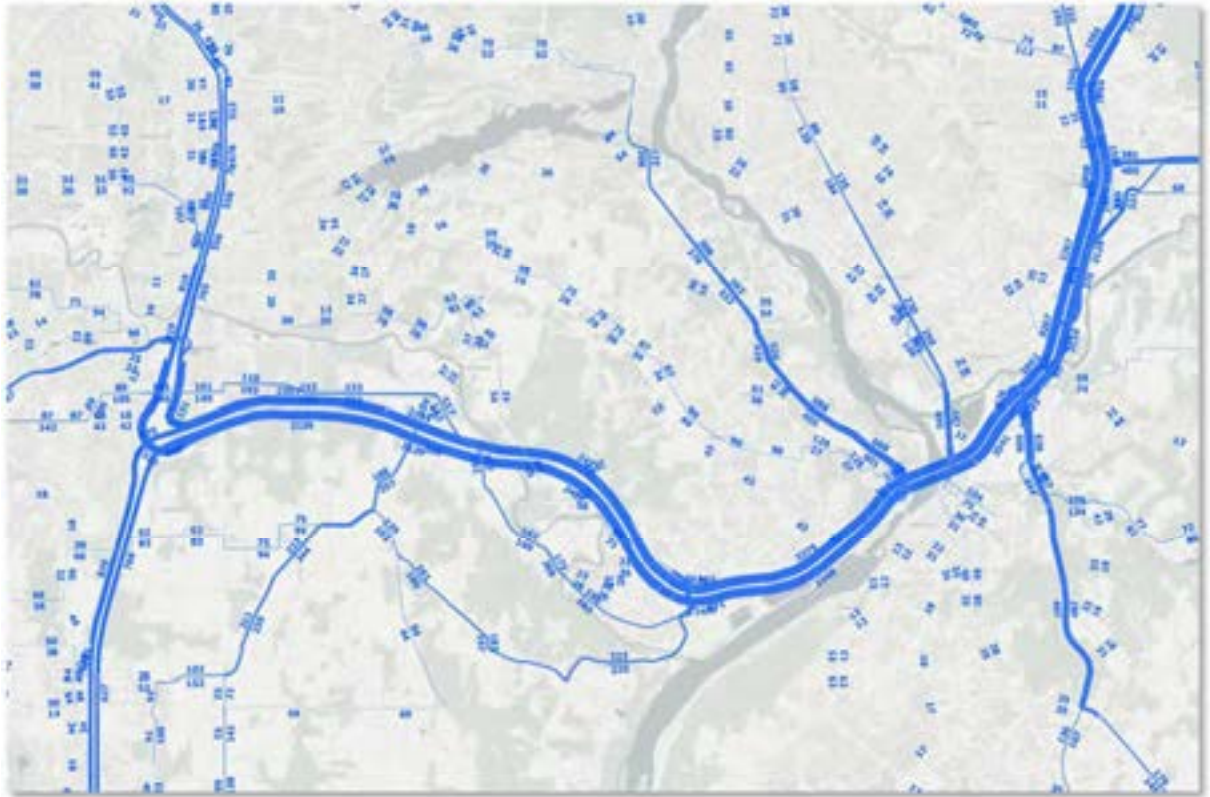
Figure 7 - Select Link Analysis for Vehicles Using the I-205 Bridge – 2045 Build PM Peak Traffic Volume
