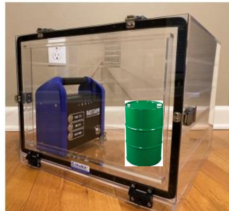
Figure A-1. Radon monitor and chamber setup.
